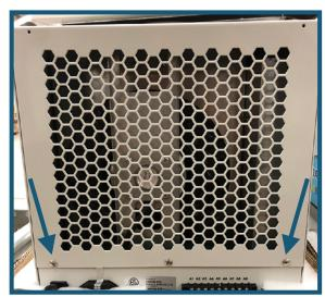
2. Place duct collar on inlet side of dehumidifier and secure with 4 screws. Repeat on exhaust side of dehumidifier, with 2 included screws and 2 saved screws.
