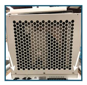
2. Place duct collar on inlet side of dehumidifier and secure with 4 screws. Repeat on exhaust side of dehumidifier, with 2 included screws and 2 saved screws.
