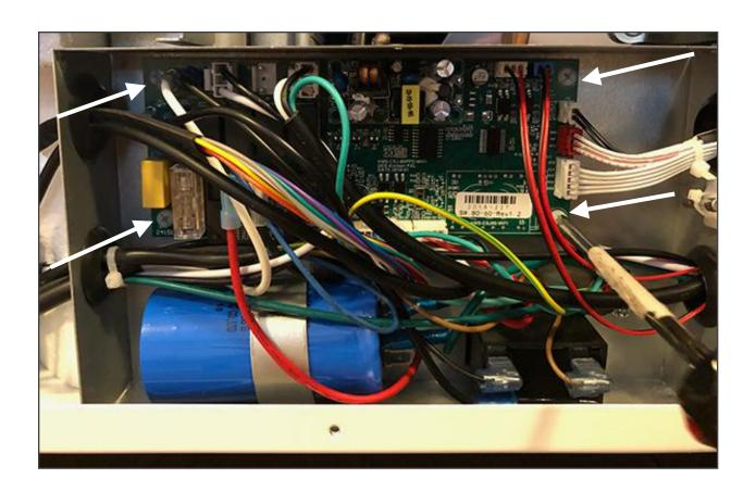
5. Finally, lift the control board out and set it aside. Insert the replacement control board and reverse the process.
