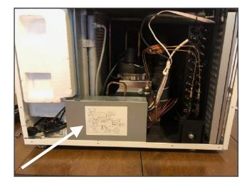
2. Remove the screw on the top of the control board cover and lift off the cover.
