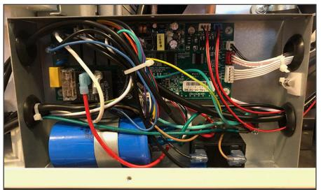
3. At this point you will need to unplug the wires from the control board.
