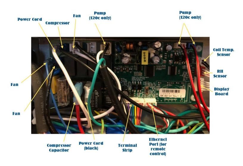
4. Next, use a screwdriver to remove the 4 screws holding the control board in place (one in each corner).
